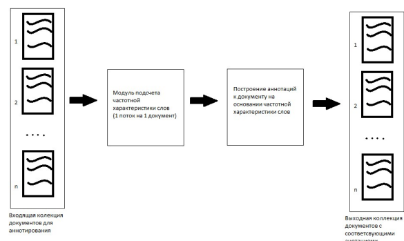
Figure 1. Simplified model of interaction of modules taking into account data decomposition for the SumBasic method.
